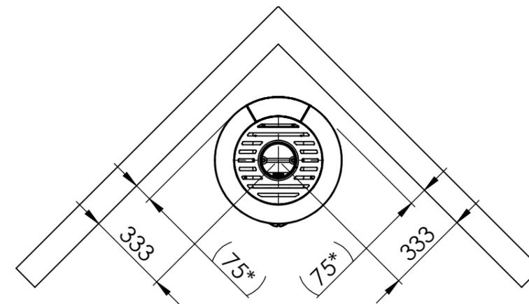
\*50 mm With insulation/ shielding of the flue gas connector (308 mm to center)
