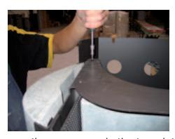
24. Remove the rear screw in the top plate.
