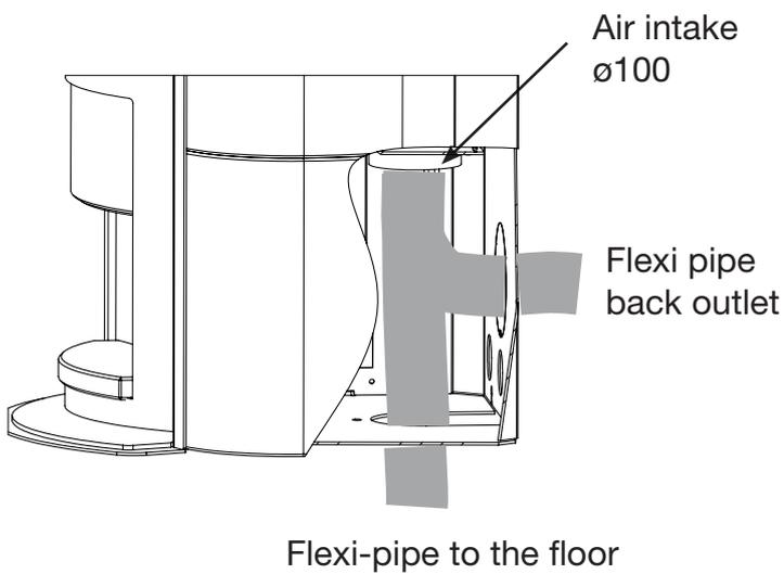
When installing external air supply, connect the air intake to the direct air pipe using flexi-pipe, both from the floor or behind the stove.
