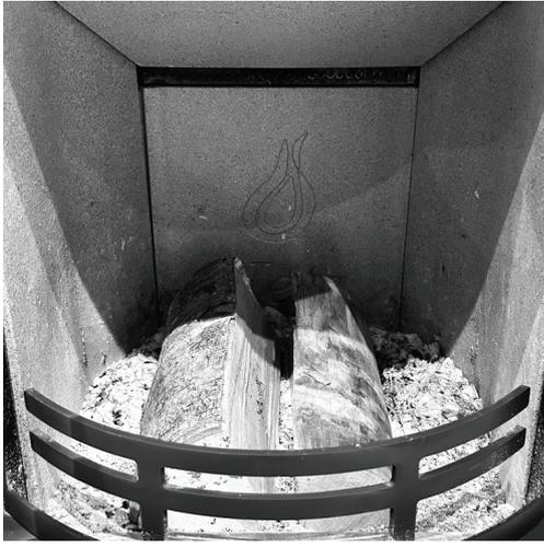
Ensure when refueling that the wood is not too close, it will cause poorer combustion, less heat out-put and lower efficiency. The fuel load, must be maintained below the top series of air holes and within the outer vent in each side. Fig. 6.
