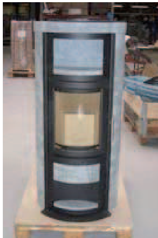
40. Installation of the Turin soapstone elements is complete.
