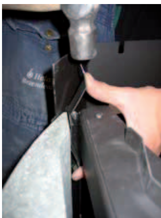
13. Install the spring for the top stone.
