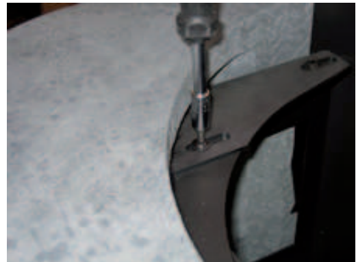
32. When the top panel is in position, tighten these screws so that it cannot move.
